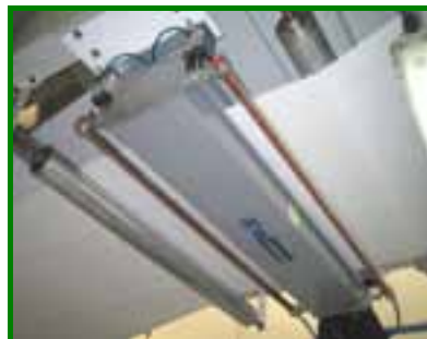
Web Cleaner DM 2000 on flexo C.I. printing press
